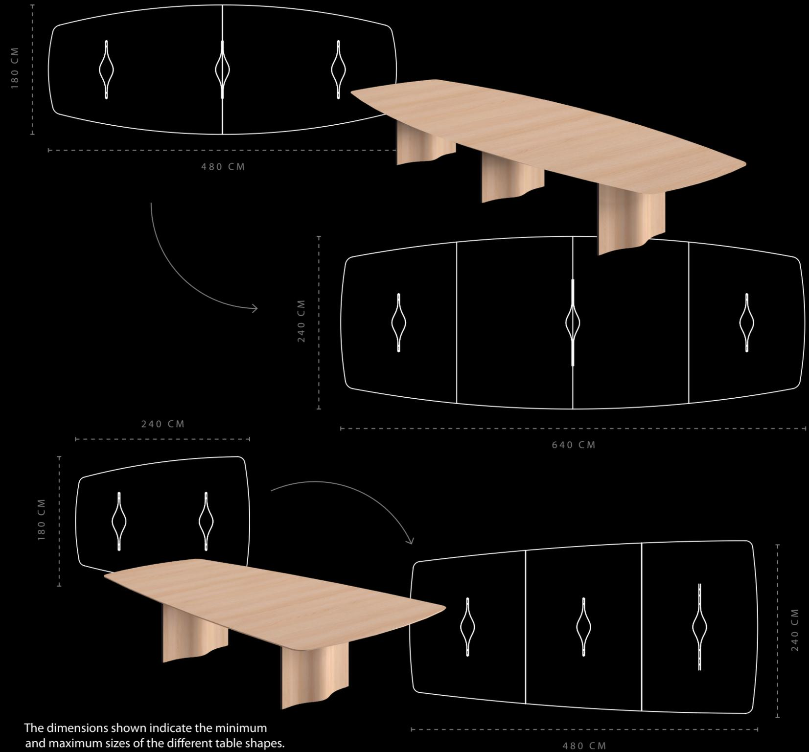
The dimensions shown indicate the minimum and maximum sizes of the different table shapes. Custom sizes on request.
